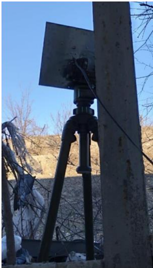
External antennas boost signal and allow drone pilots to fly from shelter
